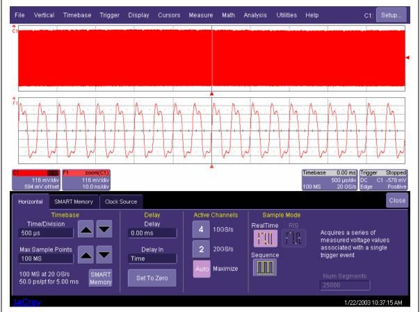
Figure 1 Timebase setup for a WaveMaster Series scope with option XXL showing the full 100 MS memory being used to acquire 5 ms of data at the maximum sampling rate of 20 GS/s
